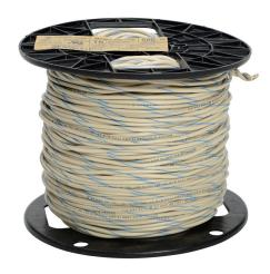
Atlas Wire MTW hook-up wire, single conductor, 18 AWG, 16-stranded, bare copper, PVC conductor insulation material, white with blue stripe, 600V, 500ft spool.
