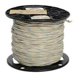
Atlas Wire MTW hook-up wire, single conductor, 18 AWG, 16-stranded, bare copper, PVC conductor insulation material, white with blue stripe, 600V, 1000ft spool.
