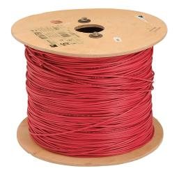
Atlas Wire MTW hook-up wire, single conductor, 18 AWG, 16-stranded, bare copper, PVC conductor insulation material, red, 600V, 2500ft reel.
