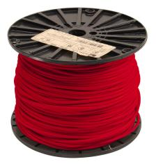
Atlas Wire MTW hook-up wire, single conductor, 18 AWG, 16-stranded, bare copper, PVC conductor insulation material, red, 600V, 1000ft spool.
