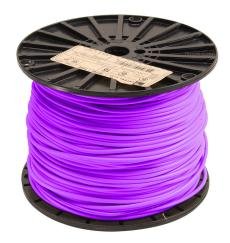
Atlas Wire MTW hook-up wire, single conductor, 18 AWG, 16-stranded, bare copper, PVC conductor insulation material, purple, 600V, 500ft spool.
