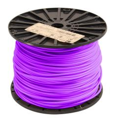
Atlas Wire MTW hook-up wire, single conductor, 18 AWG, 16-stranded, bare copper, PVC conductor insulation material, purple, 600V, 1000ft spool.
