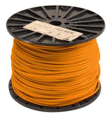
Atlas Wire MTW hook-up wire, single conductor, 18 AWG, 16-stranded, bare copper, PVC conductor insulation material, orange, 600V, 500ft spool.
