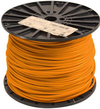
Atlas Wire MTW hook-up wire, single conductor, 18 AWG, 16-stranded, bare copper, PVC conductor insulation material, orange, 600V, 1000ft spool.
