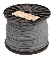
Atlas Wire MTW hook-up wire, single conductor, 18 AWG, 16-stranded, bare copper, PVC conductor insulation material, gray, 600V, 1000ft spool.
