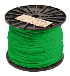
Atlas Wire MTW hook-up wire, single conductor, 18 AWG, 16-stranded, bare copper, PVC conductor insulation material, green, 600V, 1000ft spool.
