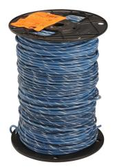
Atlas Wire MTW hook-up wire, single conductor, 18 AWG, 16-stranded, bare copper, PVC conductor insulation material, blue with white stripe, 600V, 500ft spool.
