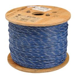
Atlas Wire MTW hook-up wire, single conductor, 18 AWG, 16-stranded, bare copper, PVC conductor insulation material, blue with white stripe, 600V, 2500ft reel.
