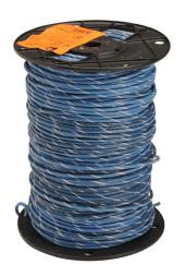
Atlas Wire MTW hook-up wire, single conductor, 18 AWG, 16-stranded, bare copper, PVC conductor insulation material, blue with white stripe, 600V, 1000ft spool.
