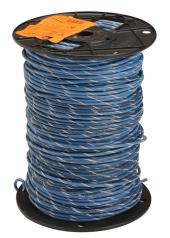
Atlas Wire MTW hook-up wire, single conductor, 18 AWG, 16-stranded, bare copper, PVC conductor insulation material, blue with white stripe, 600V, 1000ft spool.
