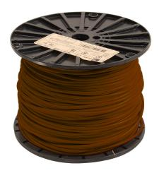
Atlas Wire MTW hook-up wire, single conductor, 18 AWG, 16-stranded, bare copper, PVC conductor insulation material, brown, 600V, 500ft spool.
