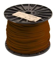
Atlas Wire MTW hook-up wire, single conductor, 18 AWG, 16-stranded, bare copper, PVC conductor insulation material, brown, 600V, 1000ft spool.
