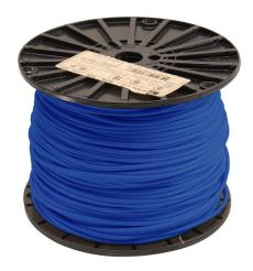
Atlas Wire MTW hook-up wire, single conductor, 18 AWG, 16-stranded, bare copper, PVC conductor insulation material, blue, 600V, 500ft spool.
