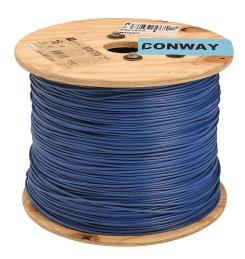
Atlas Wire MTW hook-up wire, single conductor, 18 AWG, 16-stranded, bare copper, PVC conductor insulation material, blue, 600V, 2500ft reel.
