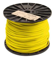
Atlas Wire MTW hook-up wire, single conductor, 16 AWG, 26-stranded, bare copper, PVC conductor insulation material, yellow, 600V, 500ft spool.
