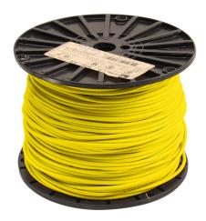
Atlas Wire MTW hook-up wire, single conductor, 16 AWG, 26-stranded, bare copper, PVC conductor insulation material, yellow, 600V, 1000ft spool.
