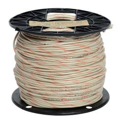
Atlas Wire MTW hook-up wire, single conductor, 16 AWG, 26-stranded, bare copper, PVC conductor insulation material, white with orange stripe, 600V, 500ft spool.
