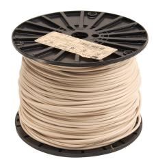
Atlas Wire MTW hook-up wire, single conductor, 16 AWG, 26-stranded, bare copper, PVC conductor insulation material, white, 600V, 500ft spool.
