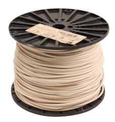
Atlas Wire MTW hook-up wire, single conductor, 16 AWG, 26-stranded, bare copper, PVC conductor insulation material, white, 600V, 1000ft spool.
