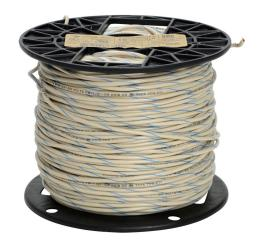
Atlas Wire MTW hook-up wire, single conductor, 16 AWG, 26-stranded, bare copper, PVC conductor insulation material, white with blue stripe, 600V, 500ft spool.
