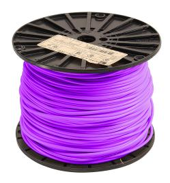
Atlas Wire MTW hook-up wire, single conductor, 16 AWG, 26-stranded, bare copper, PVC conductor insulation material, purple, 600V, 500ft spool.
