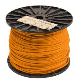
Atlas Wire MTW hook-up wire, single conductor, 16 AWG, 26-stranded, bare copper, PVC conductor insulation material, orange, 600V, 500ft spool.
