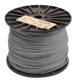
Atlas Wire MTW hook-up wire, single conductor, 16 AWG, 26-stranded, bare copper, PVC conductor insulation material, gray, 600V, 500ft spool.
