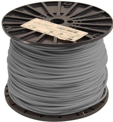
Atlas Wire MTW hook-up wire, single conductor, 16 AWG, 26-stranded, bare copper, PVC conductor insulation material, gray, 600V, 500ft spool.
