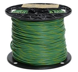
Atlas Wire MTW hook-up wire, single conductor, 16 AWG, 26-stranded, bare copper, PVC conductor insulation material, green with yellow stripe, 600V, 500ft spool.
