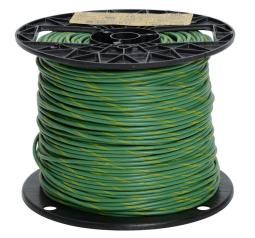
Atlas Wire MTW hook-up wire, single conductor, 16 AWG, 26-stranded, bare copper, PVC conductor insulation material, green with yellow stripe, 600V, 1000ft spool.
