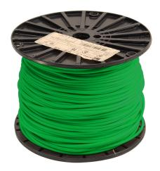
Atlas Wire MTW hook-up wire, single conductor, 16 AWG, 26-stranded, bare copper, PVC conductor insulation material, green, 600V, 1000ft spool.
