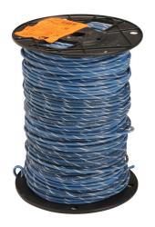
Atlas Wire MTW hook-up wire, single conductor, 16 AWG, 26-stranded, bare copper, PVC conductor insulation material, blue with white stripe, 600V, 500ft spool.
