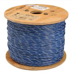
Atlas Wire MTW hook-up wire, single conductor, 16 AWG, 26-stranded, bare copper, PVC conductor insulation material, blue with white stripe, 600V, 2500ft reel.
