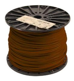
Atlas Wire MTW hook-up wire, single conductor, 16 AWG, 26-stranded, bare copper, PVC conductor insulation material, brown, 600V, 500ft spool.
