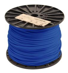
Atlas Wire MTW hook-up wire, single conductor, 16 AWG, 26-stranded, bare copper, PVC conductor insulation material, blue, 600V, 500ft spool.
