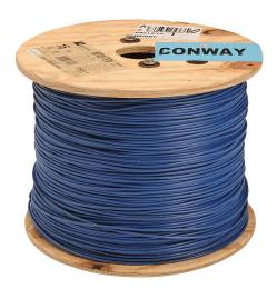
Atlas Wire MTW hook-up wire, single conductor, 16 AWG, 26-stranded, bare copper, PVC conductor insulation material, blue, 600V, 2500ft reel.
