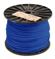
Atlas Wire MTW hook-up wire, single conductor, 16 AWG, 26-stranded, bare copper, PVC conductor insulation material, blue, 600V, 1000ft spool.
