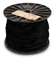
Atlas Wire MTW hook-up wire, single conductor, 16 AWG, 26-stranded, bare copper, PVC conductor insulation material, black, 600V, 500ft spool.
