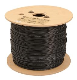
Atlas Wire MTW hook-up wire, single conductor, 16 AWG, 26-stranded, bare copper, PVC conductor insulation material, black, 600V, 2500ft reel.
