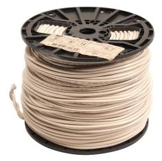
Atlas Wire MTW hook-up wire, single conductor, 14 AWG, 41-stranded, bare copper, PVC conductor insulation material, white, 600V, 1000ft spool.
