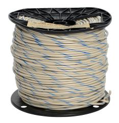
Atlas Wire MTW hook-up wire, single conductor, 14 AWG, 41-stranded, bare copper, PVC conductor insulation material, white with blue stripe, 600V, 500ft spool.
