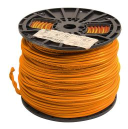
Atlas Wire MTW hook-up wire, single conductor, 14 AWG, 41-stranded, bare copper, PVC conductor insulation material, orange, 600V, 500ft spool.
