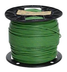
Atlas Wire MTW hook-up wire, single conductor, 14 AWG, 41-stranded, bare copper, PVC conductor insulation material, green with yellow stripe, 600V, 500ft spool.
