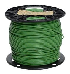
Atlas Wire MTW hook-up wire, single conductor, 14 AWG, 41-stranded, bare copper, PVC conductor insulation material, green with yellow stripe, 600V, 1000ft spool.
