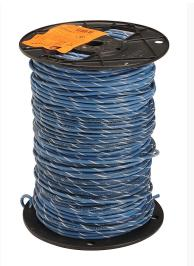
Atlas Wire MTW hook-up wire, single conductor, 14 AWG, 41-stranded, bare copper, PVC conductor insulation material, blue with white stripe, 600V, 500ft spool.
