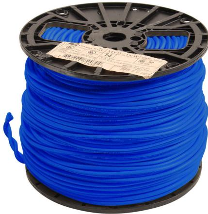
Atlas Wire MTW hook-up wire, single conductor, 14 AWG, 41-stranded, bare copper, PVC conductor insulation material, blue, 600V, 1000ft spool.
