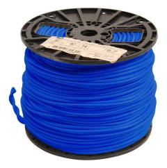
Atlas Wire MTW hook-up wire, single conductor, 14 AWG, 41-stranded, bare copper, PVC conductor insulation material, blue, 600V, 1000ft spool.
