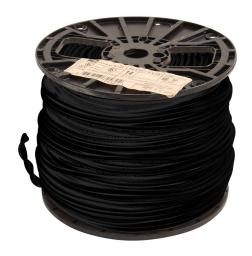
Atlas Wire MTW hook-up wire, single conductor, 14 AWG, 41-stranded, bare copper, PVC conductor insulation material, black, 600V, 500ft spool.
