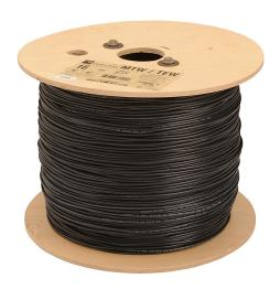
Atlas Wire MTW hook-up wire, single conductor, 14 AWG, 41-stranded, bare copper, PVC conductor insulation material, black, 600V, 2500ft reel.
