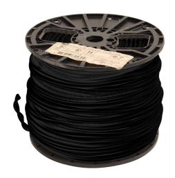
Atlas Wire MTW hook-up wire, single conductor, 14 AWG, 41-stranded, bare copper, PVC conductor insulation material, black, 600V, 1000ft spool.
