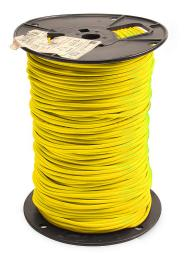
Atlas Wire MTW hook-up wire, single conductor, 12 AWG, 65-stranded, bare copper, PVC conductor insulation material, yellow, 600V, 500ft spool.
