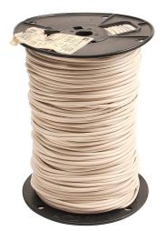
Atlas Wire MTW hook-up wire, single conductor, 12 AWG, 65-stranded, bare copper, PVC conductor insulation material, white, 600V, 500ft spool.
