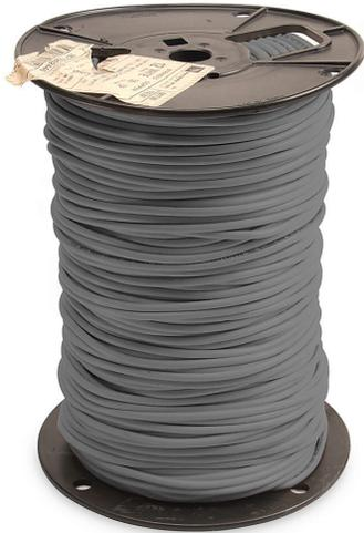
Atlas Wire MTW hook-up wire, single conductor, 12 AWG, 65-stranded, bare copper, PVC conductor insulation material, gray, 600V, 500ft spool.
