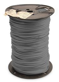
Atlas Wire MTW hook-up wire, single conductor, 12 AWG, 65-stranded, bare copper, PVC conductor insulation material, gray, 600V, 500ft spool.
